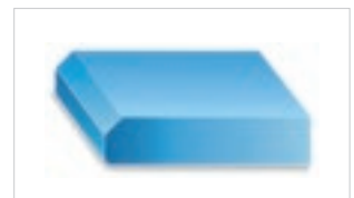
Flat edge with increased 45° chamfer.
